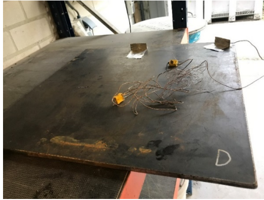
Figure 2B - Image showing the position of thermocouples on the slab
