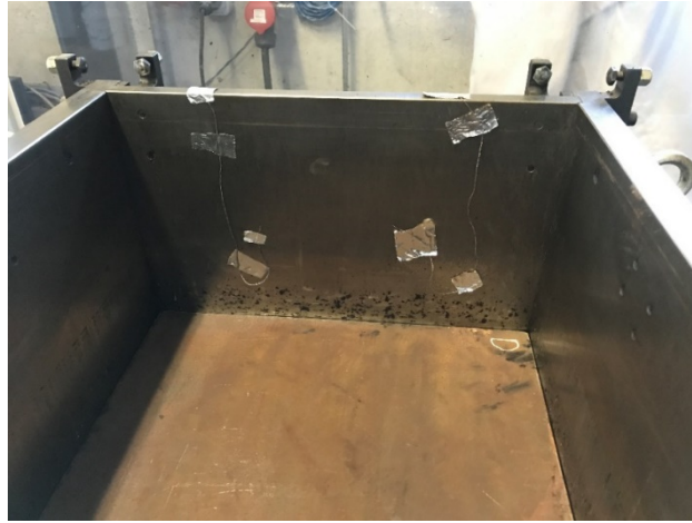
Figure 3B - Image showing the position of thermocouples on the mould
