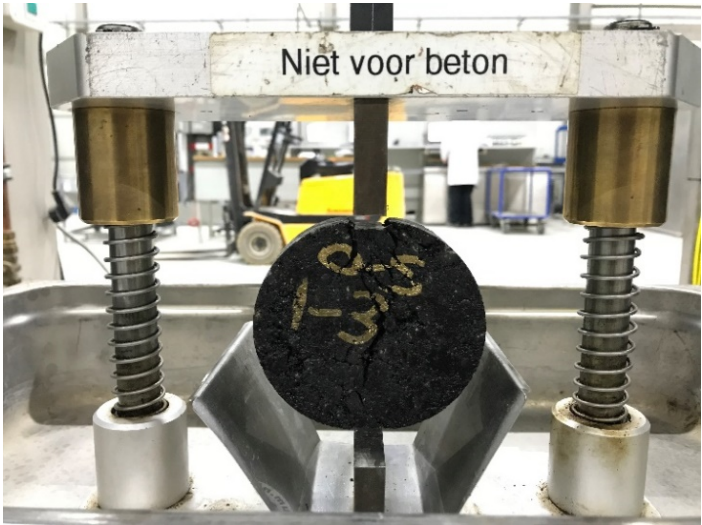
Figure 12 - One of the samples being tested in a ITS test setup.
