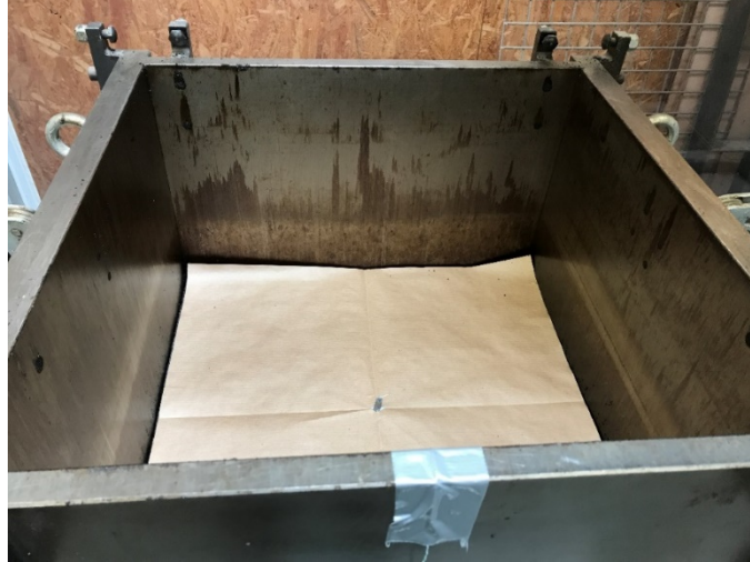
Figure 4B - Image showing the position of thermocouples on the base slab
