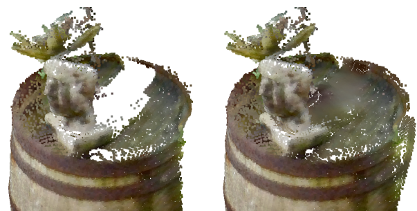
Figure 7. An example of a large occlusion hole surrounded by poorly sampled colors in the Backyard segment. The colors of the input (left) are smoothly interpolated in the inpainting result (right). The bust visible in the image was processed separately. Points in the background have been removed for visual clarity.
