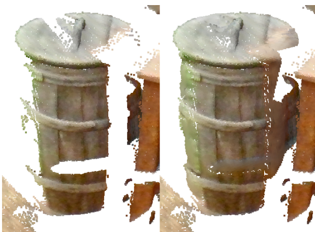
Figure 6. A close-up view of input (left) and output (right) point cloud of a wooden barrel in the Backyard segment. Note how both the shape and colors of the generated surfaces match the surrounding scan.
