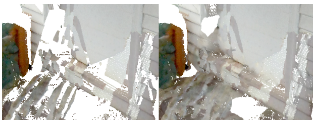
Figure 5. Inpainting the Backyard segment. Even though the input data (left) is of low quality, a plausible surface can be inferred in the output (right) point cloud.
