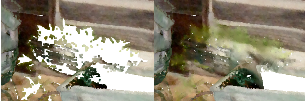
Figure 8. Color leaks in the Stairs segment. The input point cloud (left) has greenish tint around the occluded region because of projected colors captured by the RGB camera. In the inpainting result (right) the same tint has been propagated to the generated regions.
