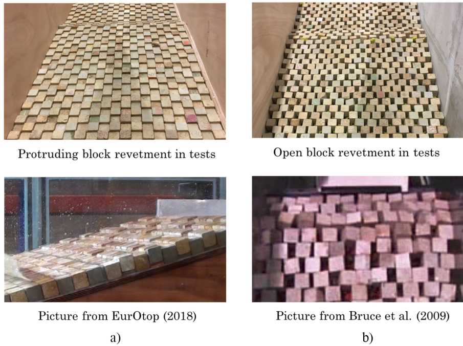
Fig. 5. Comparison of rough slopes with those provided in previous literature with a) protruding block revetment and b) open block revetment.
