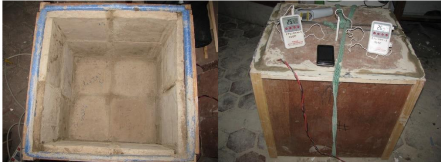
Figure 3: Testing of the insulation tile in thermo box.
