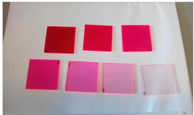
Fig. 6. Different colours result from different dye concentration using Lumogen Red 305. The concentrations are from top left to bottom right: 500, 184, 127, 97, 35.5, 15.5 and 4 ppm.
