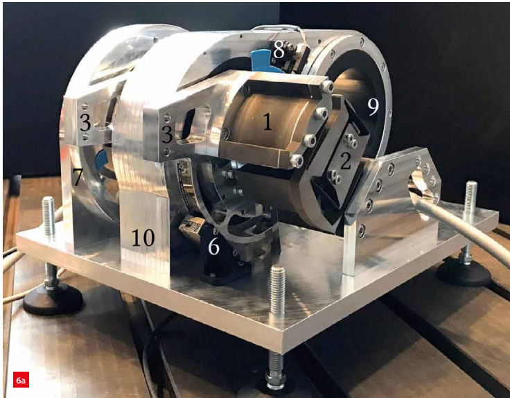
The assembled flexure-based actuator suspension, with 1) butterfly hinge, 2) slaving mechanism, 3) rotor hub, 6) encoder, 7) mechanical stop, 9) actuator's stator, and 10) stator housing. (a) Overview. (b) Trimmed view, with the torque motor and stator housing removed.
