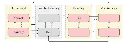
**Fig. 3.** A simplified visual representation of the FSM. The two transitions that are later written-out as pseudo code in Fig. 4 are labelled A and B.
