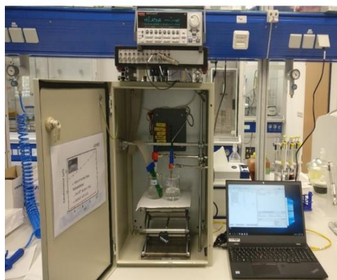
Figure S13.1 (LEFT) pH measurements set-up with the Faraday cage, the PCB with the chip immersed in the buffers connected to the switching box and the Keithley sourcemeter used for the electric measurements.
