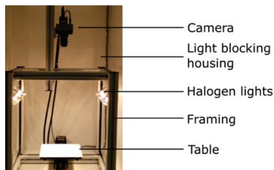
Fig. 2. The imaging system used to collect the HSI data. Tissue is placed on the Table in the bottom. The Table shifts the tissue under the sensor.
