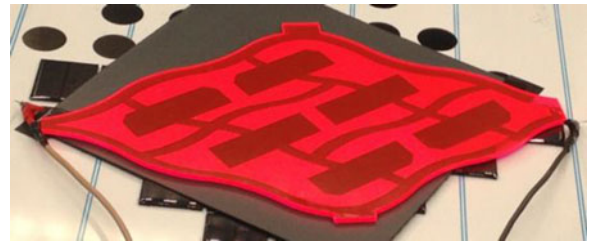
Fig. 2. Prototype of a recently developed new design for LSC PV elements, entitled Leaf Roof [10].
