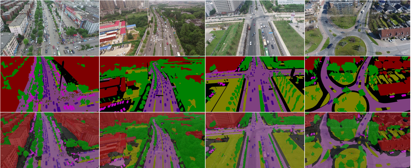
Fig. 1. Example images and labels from UAVID dataset. First row shows the images captured by UAV. Second row shows the corresponding ground truth labels. Third row shows the prediction results of MS-Dilation net+PRT+FSO model as in Tab. I.
