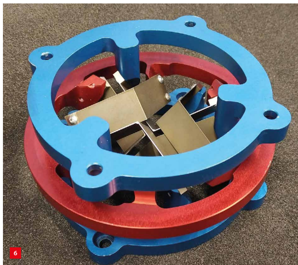
Two views of a realisation of the SFL-flexure joint. Diameter of the red intermediate body is 140 mm and the height of the joint is 70 mm.
