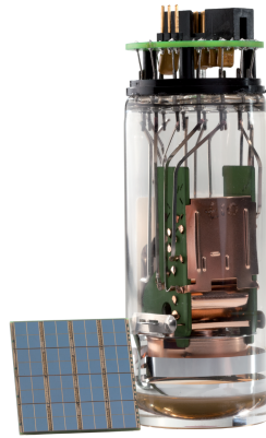
Figure 1 Digital silicon photomultiplier (left) and conventional photomultiplier tube (right). The digital technique results in a better timing resolution and higher photon detection efficiency. Adapted from [44], images courtesy of Philips Healthcare
