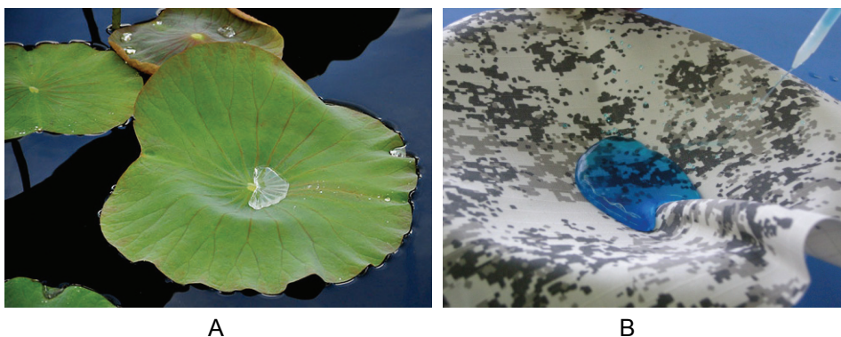
Figure 21. A leaf of the lotus flower Nelumbo nucifera (A) and the cotton woven fabric with the “Lotus-Effect” (B).
