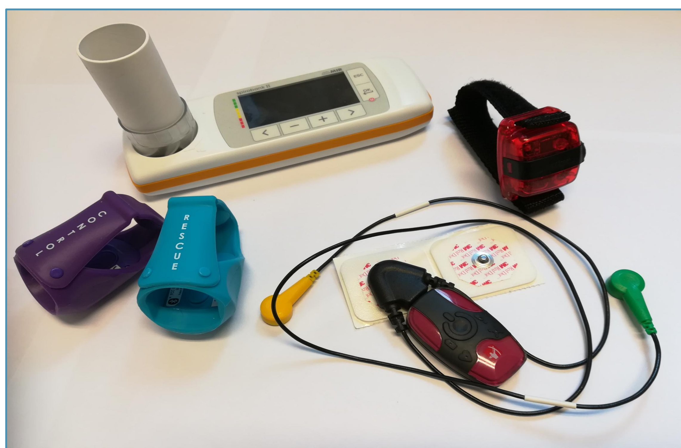
Figure 1: Smart devices from top-left to bottom-right: Spirobank II, Actigraph wGT3X-BT, Cohero Health smart inhalers, eMotion Faros 180.
