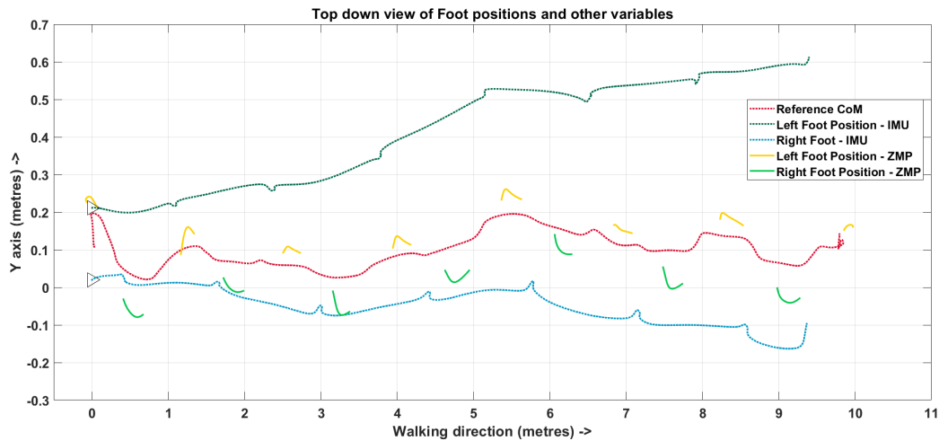
Fig. 3. Different trajectories from the example with IMUs in Section II-E are plotted. The dark green dotted line and blue dotted lines are the left and right foot trajectories respectively, estimated from the algorithm of Weenk et al [10] from the foot IMUs. The red dotted line is the reference centre of mass (CoM) estimated by the ForceShoe TM . The solid yellow lines are possible estimates for left foot during right swing phase, and solid green lines are possible estimates for the right foot during left swing phase. These are estimated using the CoM and zero moment point assumptions. The triangles denote the starting position of the two feet.
