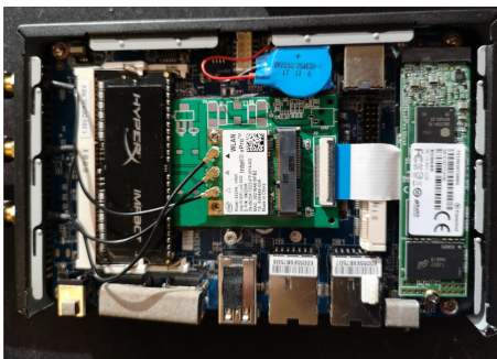
Figure 1: Inside of the Gigabyte Brix IoT (receiver node) with the Intel 5300 NIC
