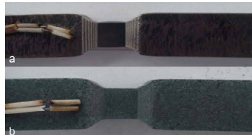
Figure 3. Two specimens, subjected to a) 15 'strong' hits and b) 80 'shallow' hits.
