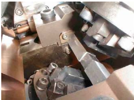
Figure 1. Gleeble MAXStrain multi-axis deformation system showing specimen and anvils (courtesy Dynamic Systems Inc.).
