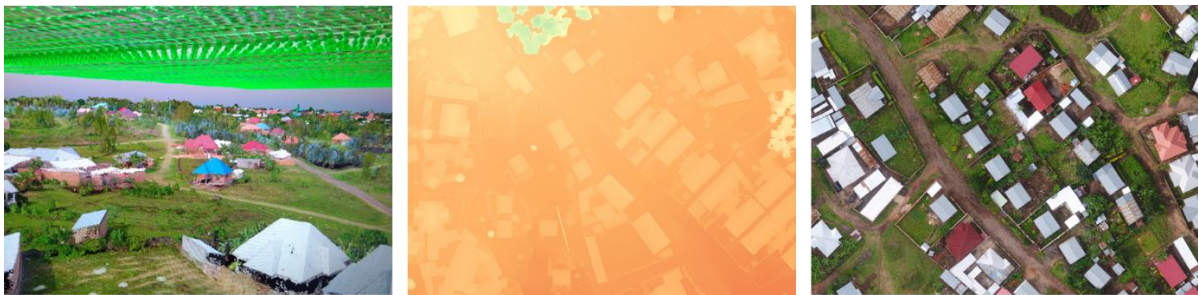
Figure 4: Data products derived from UAV images. left: 3D point cloud; centre: digital surface model; right: orthophoto
