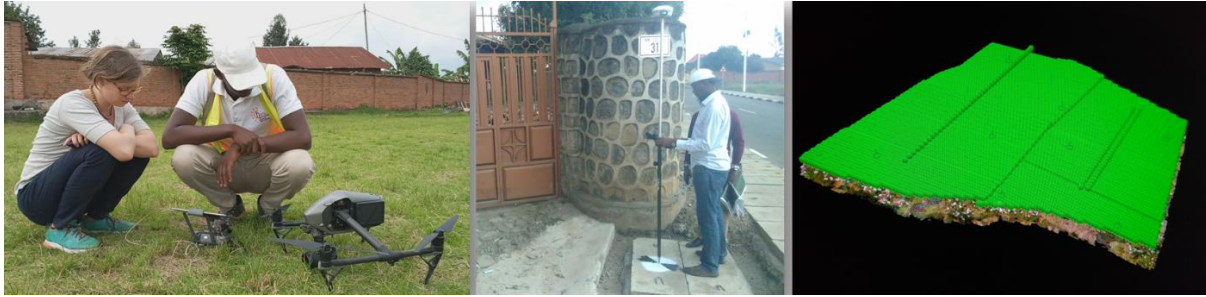
Figure 2: UAV data collection. left: checking the UAV DJI Inspire Pro before the flight; centre: measurement of ground control points for georeferencing; right: data processing in Pix4D
