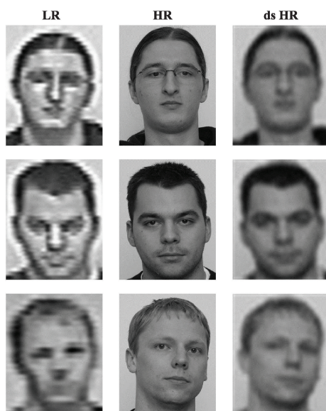
Fig. 2 LR Challenges in Surveillance Applications: LR has been a long-standing problem in face recognition in surveillance scenarios. From left to right, these figures show LR, HR, and downsampled HR (ds HR) images. 'LR' images are captured from surveillance cameras. 'HR' images are taken under controlled conditions. 'ds HR' images are downsampled from HR images to the same resolution as 'LR'. Obvious differences can be observed in appearance between the three types of images
