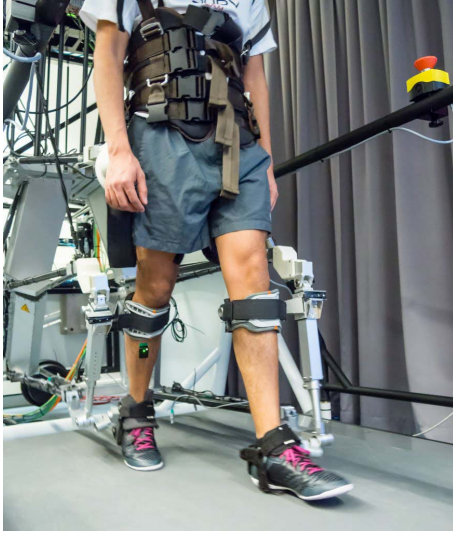
Fig. 2. A subject walking with LOPES II exoskeleton.
