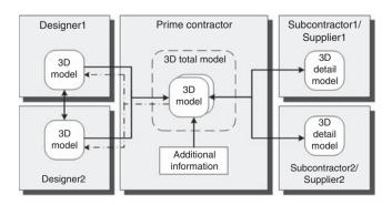
**Figure 2.** Data exchange using BIM
