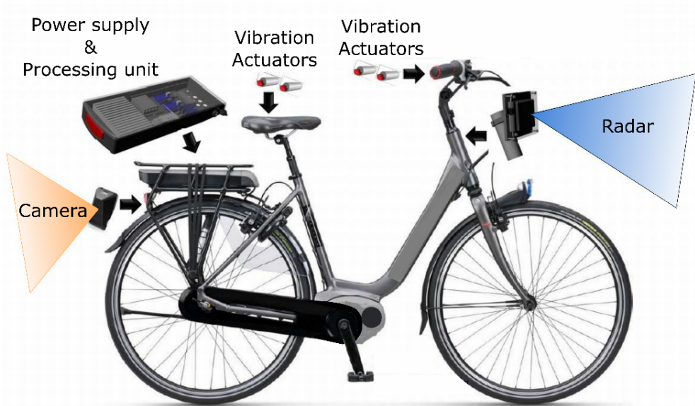
Figure 1. Instrumented bicycle with components that was used during the experiment.
