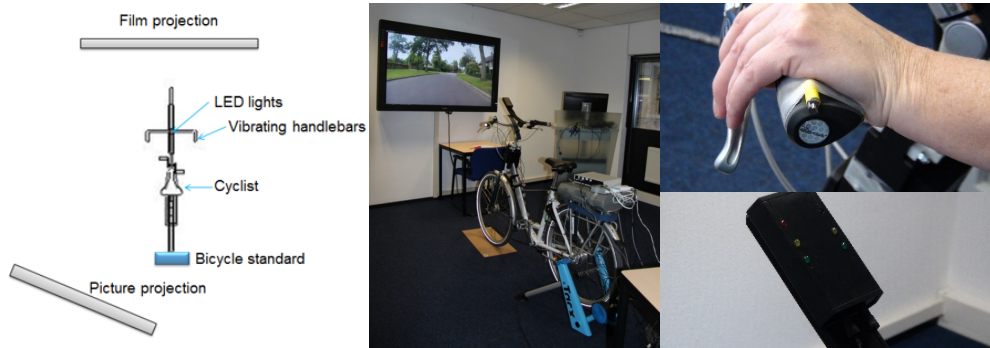
Figure 1. Experimental set-up. On the left a schematic overview, and on the right a close up of the vibrating handles and the LED display.
