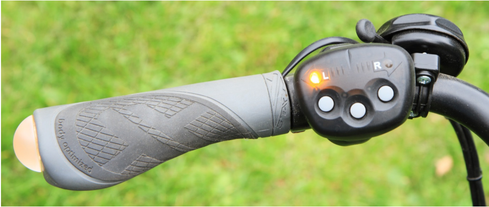
Figure 4. The remote control unit mounted on the left-hand side of the handlebars.
