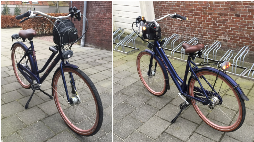
Figure 3. The instrumented bicycle with activated indicators that was used in the experiment.
