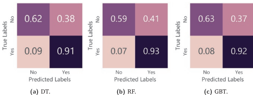
Figure 5.6: Confusion matrices of maintenance need prediction on held-out test set.
