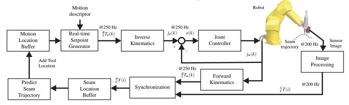
Figure 1: Trajectory-based control architecture
