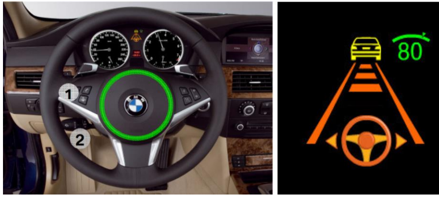
Figure 2: BMW's interface for Traffic Jam Assist. An additional feature shown in (a) consists of an illuminated ring on the steering wheel to provide feedback on system status. Picture (b) shows the standard interface. (Picture: adopted from Schaller [17])
