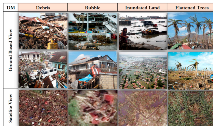
Figure 7. Illustration of damage classes, both ground and satellite views; DM: Damage class, sources: Satellite view from World-View2 and Google Earth; ground-based view from Google Street View, Flickr, Wikipedia, Wikimedia.
