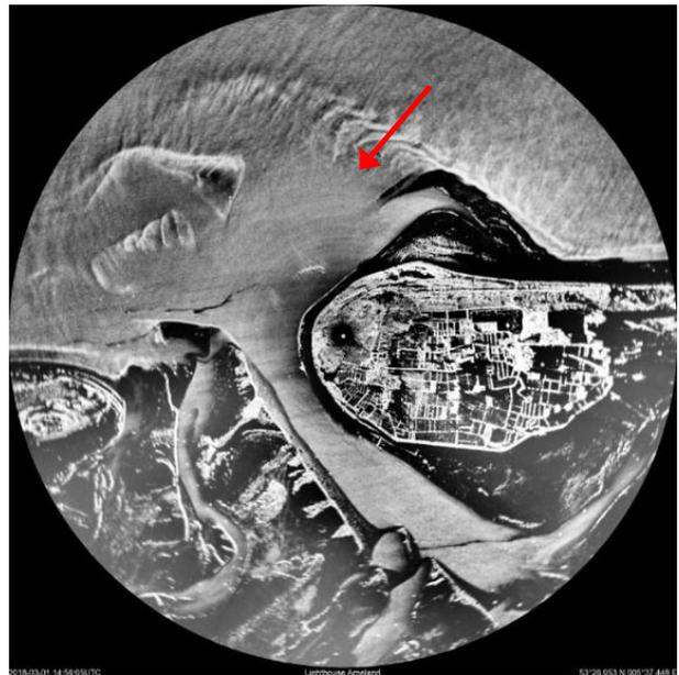
*Fig 2: Averaged radar image of the Ameland inlet. One of the ice patches is indicated with a red arrow.*
