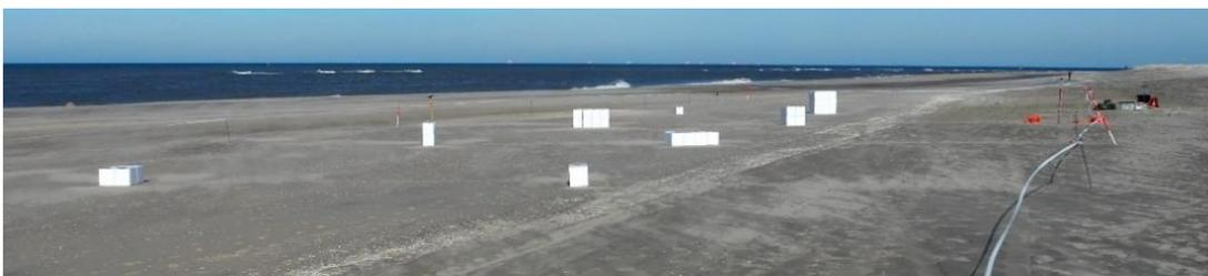
Figure 1: Photo of one of the set-ups, testing the effect of building width and height in October 2018
