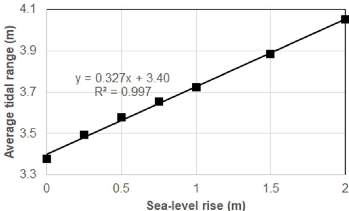
Figure 1 Simulated spatially average tidal range in the Oosterschelde in the SLR scenarios. The line denotes the linear regression between the average tidal range and SLR amplitude.
