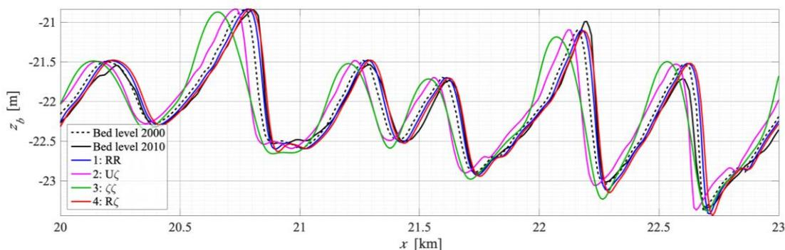
Figure 1. Bed level  $z_b$  measured in 2000 and 2010 (dashed and solid black lines, respectively) over  $x$ , and simulated  $z_b$  for the different types of boundary conditions: 1. two Riemann invariants (RR, blue); 2. depth-averaged velocity and water level time series ( $U\zeta$ , magenta); 3. two water level time series ( $\zeta\zeta$ , green); 4. Riemann invariants ( $R\zeta$ , red).
