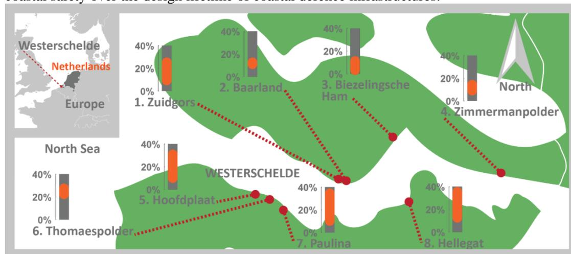
Figure 1. Minimum wave attenuation for eight foreshores in the Westerschelde. The minimum wave attenuating capacity of every transect is summarized per foreshore (orange bar).
