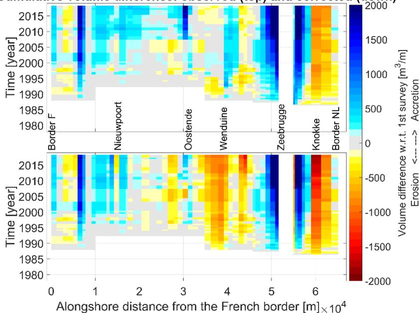
Figure 1 Time stack of cumulative volume differences along the Belgian coast. Cold colours indicate accretion, warm colours erosion. Top panel: observed values, bottom panel: after corrections for artificial works.
