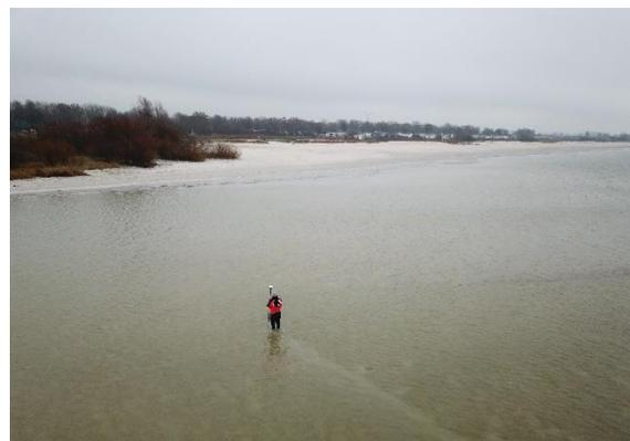
Figure 1. Left: cross-shore profile taken at Broekerhaven, one of the study sites in the Markermeer. Right: measuring beach cross-shore profile with hand-held GPS in the IJsselmeer.
