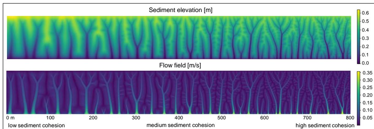
Figure 1 Top view on simulated drainage topography (m) and flow speeds (m/s) along a gradient of (to the right) increasing sediment cohesion. Outflow occurs through the lower boundary; the other boundaries are closed.
