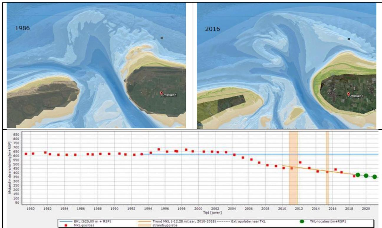
Figure 1 Example of large scale changes: bed topography in the Ameland Inlet System (top: 1986 and 2016) and the (calculated) coastline position in a transect at Ameland (TKL) (below).
