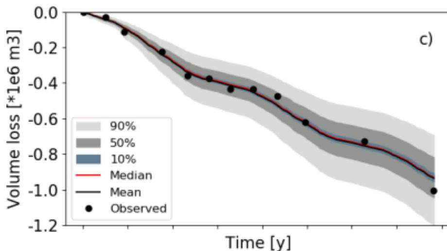
Figure 1 Stochastic forecast of volume loss compared to observed volume loss for the period of June 2015 to January 2018.
