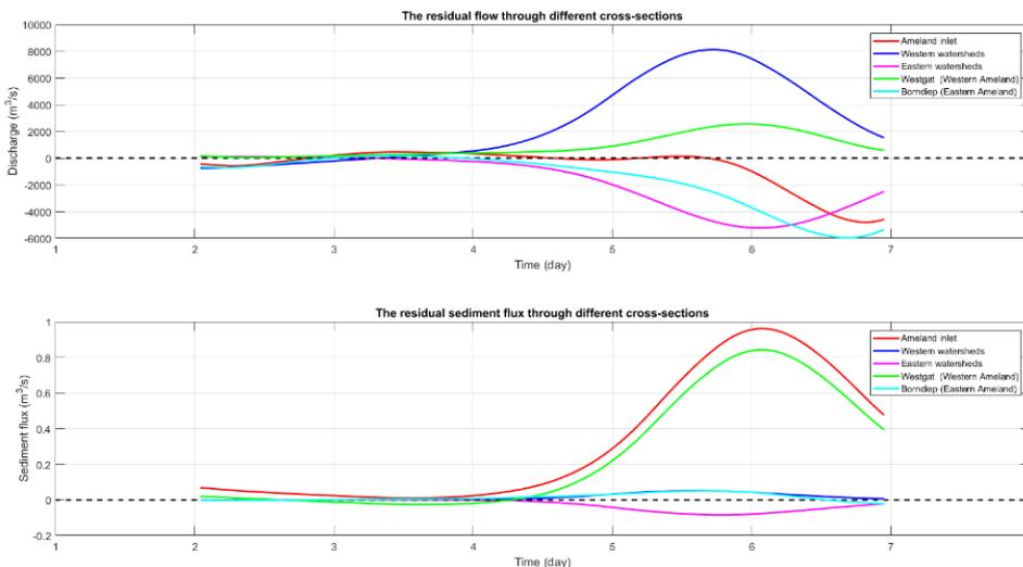
Figure 1 The time-series of residual flow and sediment transport through 5 cross-sections of Ameland Inlet.
