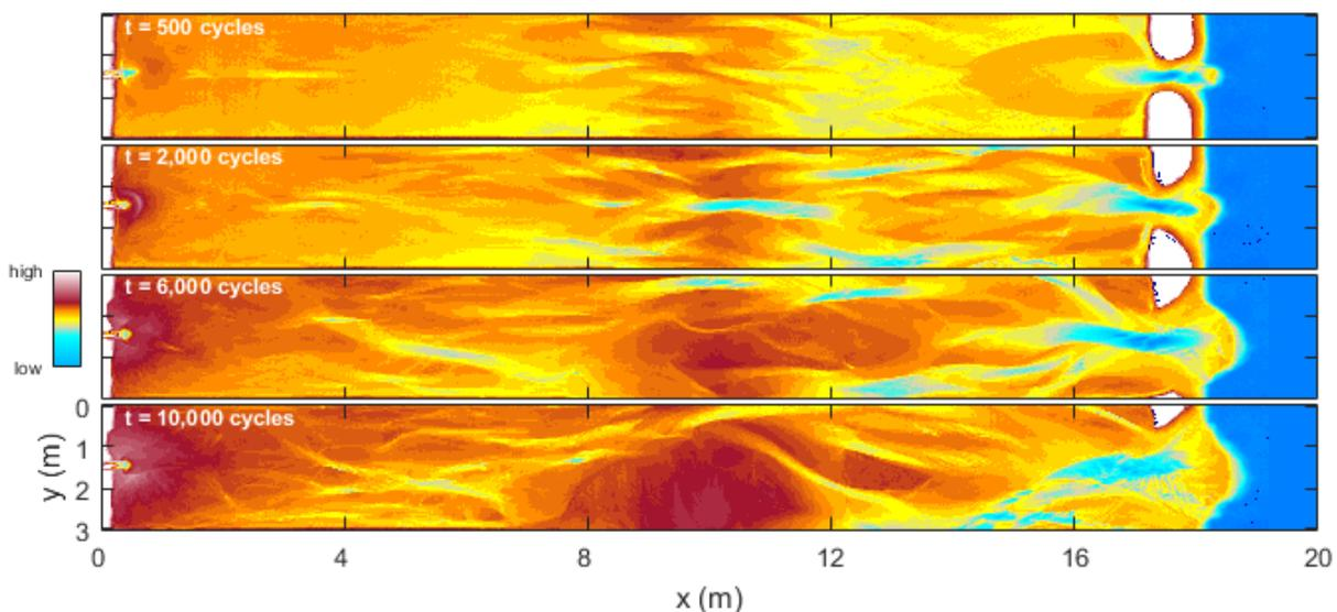
Figure 1 Morphological development of experiment sand+mud. Elevation is not yet calibrated.
