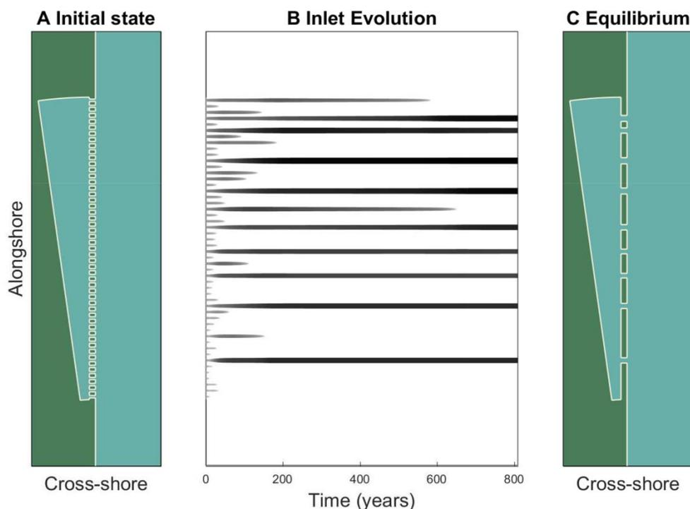
Figure 1: Example run showing the evolution of a barrier coast from a saturated coast with many open inlets (A), evolving over time (B) towards an equilibrium state with 9 open inlets (C).
