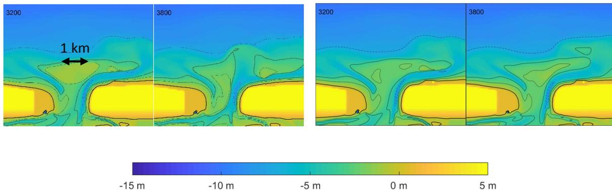
Figure 1. Depth obtained in model simulation with (left) and without (right) nourishment at the updrift shoal at the moment of nourishment placement (3200 modeled days) and 600 days hereafter. It can be seen that the nourished ebb-tidal delta is close to shoal attachment and new channel has formed, whereas the base case is still in the preceding phase of channel rotation and shoal growth.
