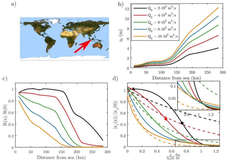
Figure 1: Location of the Kapuas Delta in Indonesia (a), Observed tidally averaged water level (b) and tidal admittance (c) along the Kapuas River, tidal admittance as predicted with a conventional model that ignores the bed slope (d, dashed) and by the extended model that incorporates backwater effects (d, solid)
