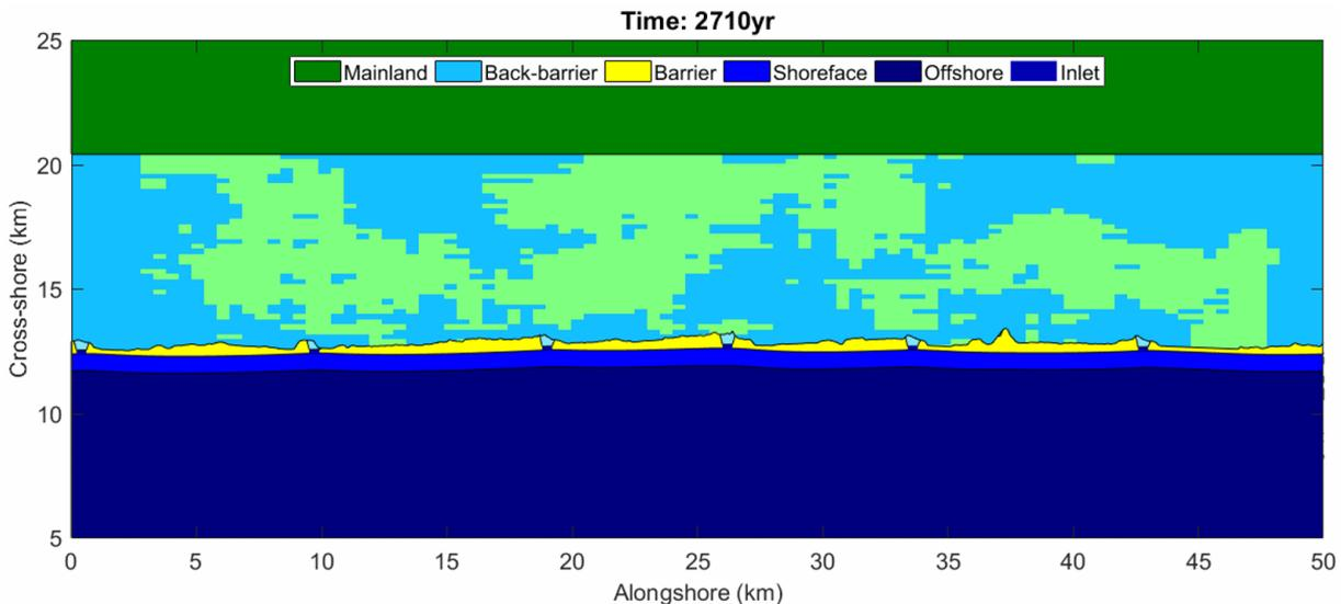
Figure 1: BRIE model showing inlets along a barrier island chain.
