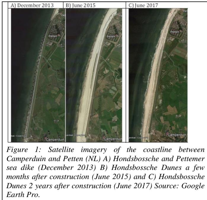
Figure 1: Satellite imagery of the coastline between Camperduin and Petten (NL) A) Hondsbossche and Pettemer sea dike (December 2013) B) Hondsbossche Dunes a few months after construction (June 2015) and C) Hondsbossche Dunes 2 years after construction (June 2017) Source: Google Earth Pro.
