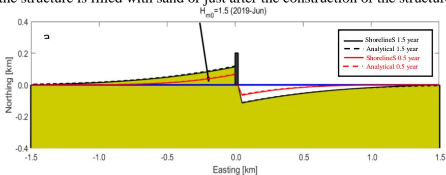
Figure 1. ShorelineS result compared to Pelnard-Considère analytical solution near a single groin.
