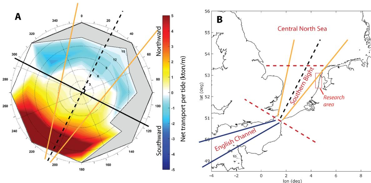
Figure 1. A. Median per wind sector of the net transport per tide (radial distance is wind speed). There is no data for the grey part. On top of the graph the orientation lines from the Southern Bight are sketched. B: Map and sketch of the English Channel – Southern Bight - Central North Sea orientation, along with the research area.
