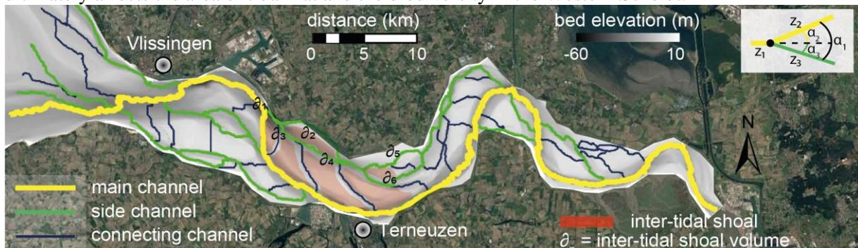
Figure 1 Extracted channel network and intertidal shoal volumes for the Western Scheldt. Right top corner shows how the bifurcation asymmetry is measured, the example indicates a symmetric bifurcation, in which the angle and bed elevation among branch 2 and 3 is equal.
