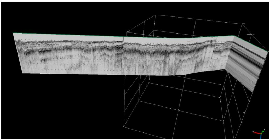
Figure 1 Example of a scanned seismic section (top) and corresponding SEG-Y transformed image.
