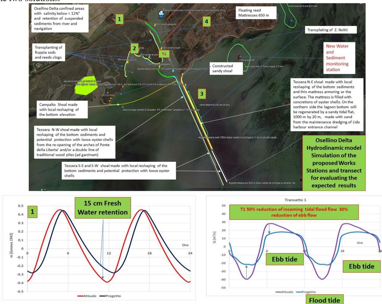
Figure 1 The retention structures at the Osellino Delta and the effects on water levels.
