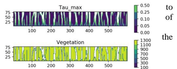
Figure 2: Resulting maximum bed shear stress and vegetation density using the Dynamic Vegetation Module
