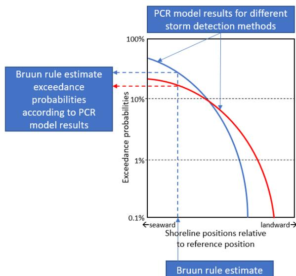
Figure 1. Explanation of the comparison of Bruun rule estimates with PCR model results. The example shown are hypothetical results of a PCR model and Bruun rule calculation for one site for one SLR scenario for one particular year.
