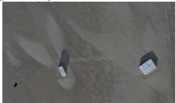
Figure 2: Digital elevation model (left) and orthophoto (right) of the sedimentation pattern around two of the models in figure 1. Model size 32x100x70 cm (left model) and 128x100x35 cm (right model).
