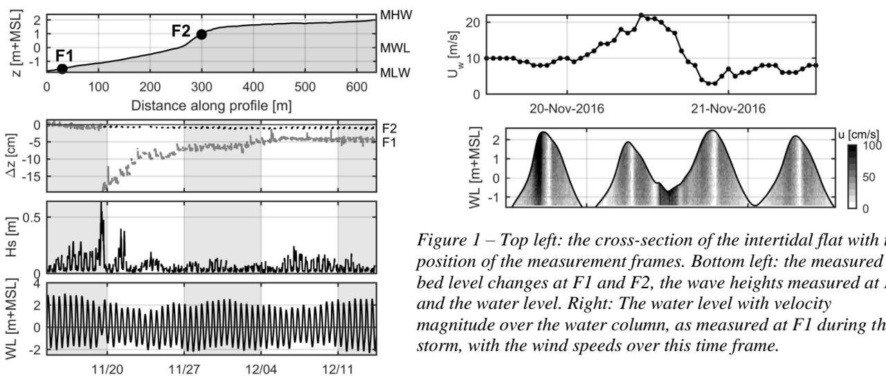
*Figure 1 – Top left: the cross-section of the intertidal flat with the position of the measurement frames. Bottom left: the measured bed level changes at F1 and F2, the wave heights measured at F1 and the water level. Right: The water level with velocity magnitude over the water column, as measured at F1 during the storm, with the wind speeds over this time frame.*
