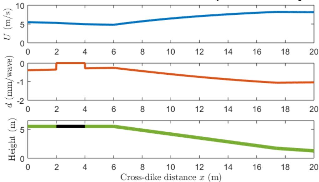
Figure 1: The flow velocity  $U$ , the erosion depth  $d$  and the cross-dike profile. The dike is covered in grass (green) with a road on the crest (black) and a transition in slope steepness around  $x=17.5$  m.
