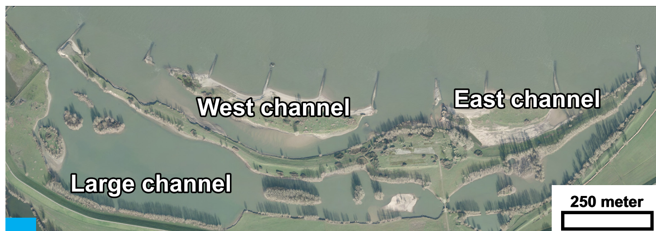
FIG. 1 An overview of the constructed side channels in the Rhine branches with a detail of the side channel system at Gameren in the river Waal. (after images of Rijkswaterstaat and Google Earth)
