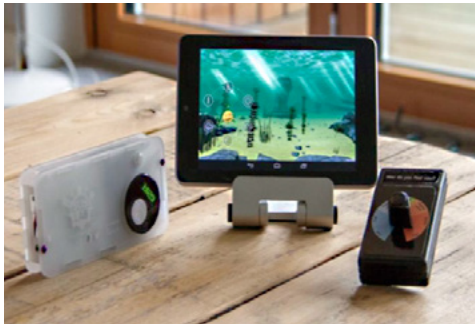
Figure 1: Data collection methods (SB=sensor box, CD=comfort dial)
