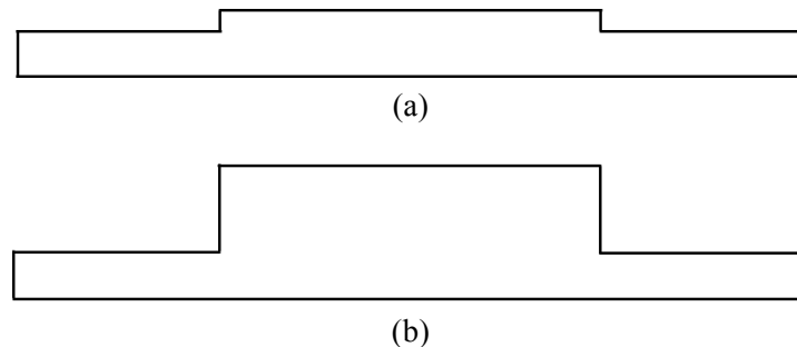
Figure 3. Pocket depth analyzed (a) h_d = \frac{1}{2} h_o (low texture depth), (b) h_d = 2 h_o (high texture depth).
