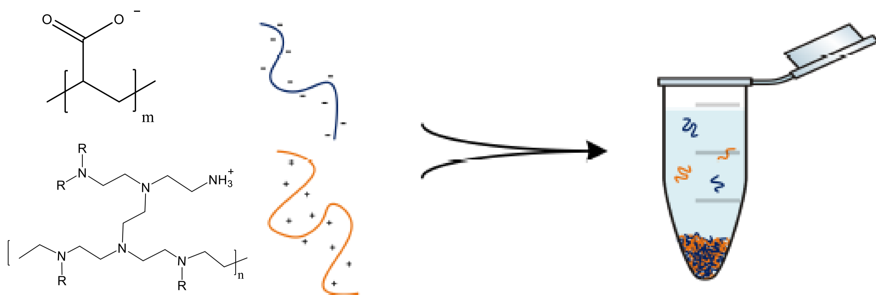
Figure 1: A schematic representation of the formation of complex coacervate with polyacrylic acid and (branched) polyethyleneimine.
