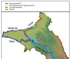
Figure 1. 1D-2D coupled hydraulic model used to perform the Monte Carlo analysis
