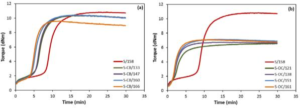
**Figure 3.** Effect of secondary fillers on cure characteristics of silica-filled NR compounds: (a) carbon black, and (b) organoclay.Dump temperatures indicated in curve designations.
