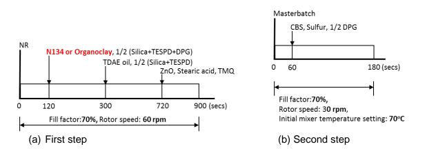
Figure 1. Two-step mixing procedure for preparing the compounds in this study.
