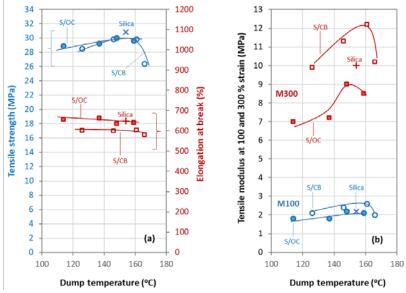
**Figure 4.** Influence of dump temperature on: (a): tensile strength and elongation at break; and (b): tensile moduli of the silica-filled NR compounds containing different secondary fillers: carbon black or organoclay.
