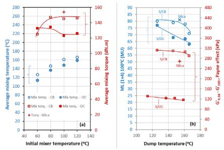
**Figure 2.** Average mixer dump/discharge temperature and torque at the final stage of mixing in the internal mixer as a function of initial mixer temperature setting. Influence of dump temperature on viscosity and Payne effect of silica-filled NR compounds with different secondary fillers: (a) carbon black and (b) organoclay.
