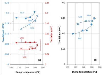
**Figure 5.** Influence of dump temperature on: (a): tan delta at -20 and 0°C from DMA; and (b) tan delta at 60°C from RPA of silica-filled NR compounds containing different secondary fillers: carbon black or organoclay.
