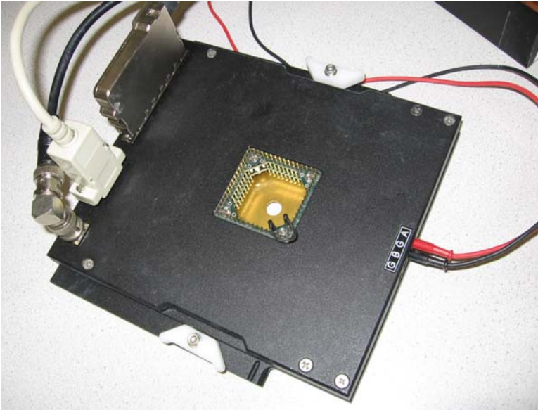
Fig. 17 Measurement set-up in which the MEA is connected to the computer while culturing conditions are controlled
