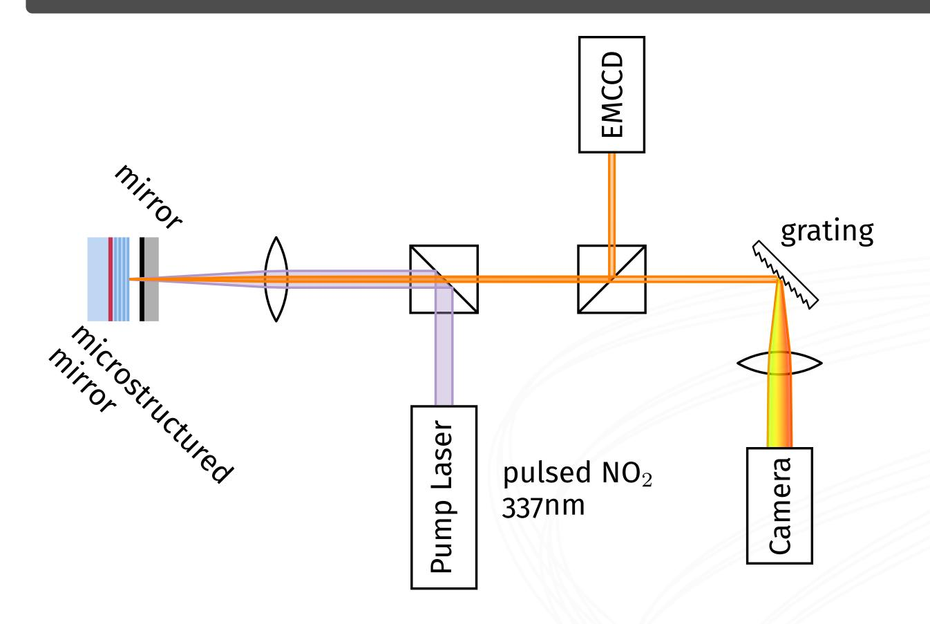
Such microstructured mirrors can be paired with a flat mirror to construct an array of microcavities. Filling the gap with Rhodamine dye and optically pumping with a pulsed UV laser forms photon Bose-Einstein condensates [1] in each microcavity. The BECs from adjacent microcavities interact via tunneling, with coupling constants [2] determined by the previous microstructuring, enabling us to arbitrarily choose the coupling constant between each BEC.
