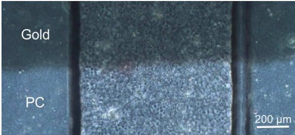
Supplementary Fig 1 The semi-transparent gold electrodes in the gut-on-a-chip device allow microscopic inspection of the Caco-2 cells cultured between them.
