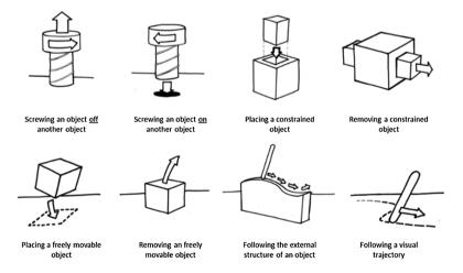
Fig. 1. Basic tasks included in our library for the remote Inspection, Repair and Maintenance use case.
