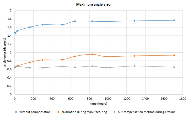
Fig. 2: Remaining angle error in a commercial sensor
