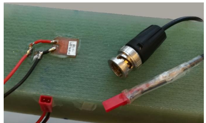
Figure 2: Composite beam with a female BEC connectors and piezoelectric transducers of PI ceramic. The coax cable with the male BEC connector is also shown.
