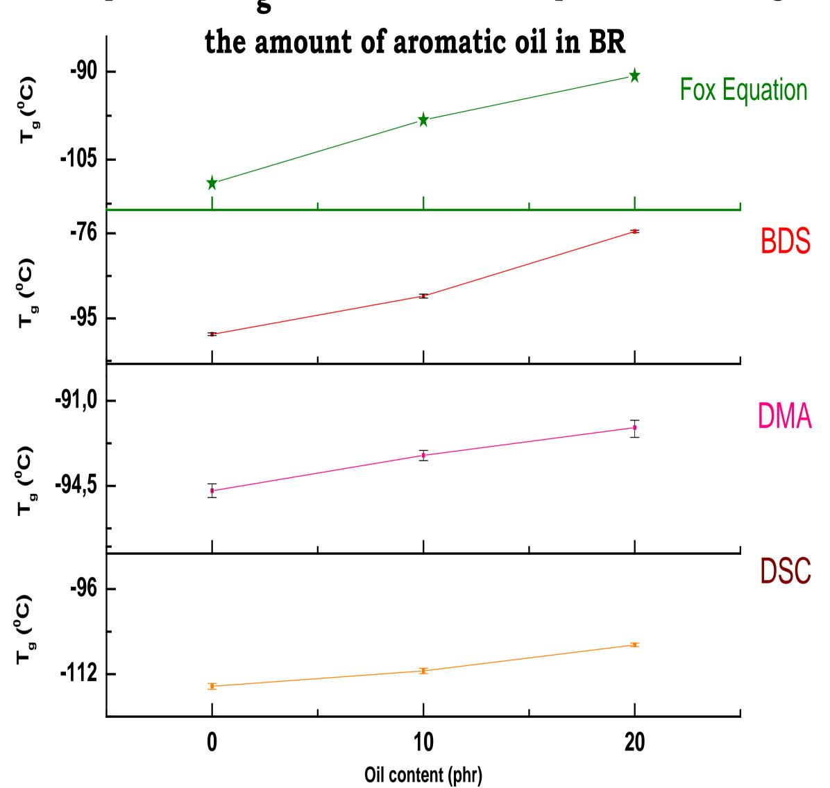
$\Box$  An advanced version of the **Fox equation**<sup>1</sup> is used to calculate the T<sub>g</sub> of oil-extended rubber.
