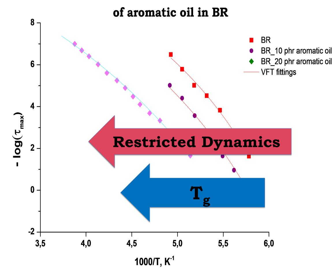
NOTE: Fittings of the data points on the graph above are done using Vogel-Fülcher-Tamman (VFT)<sup>3</sup> equation, which governs the temperature dependency of relaxation times.
