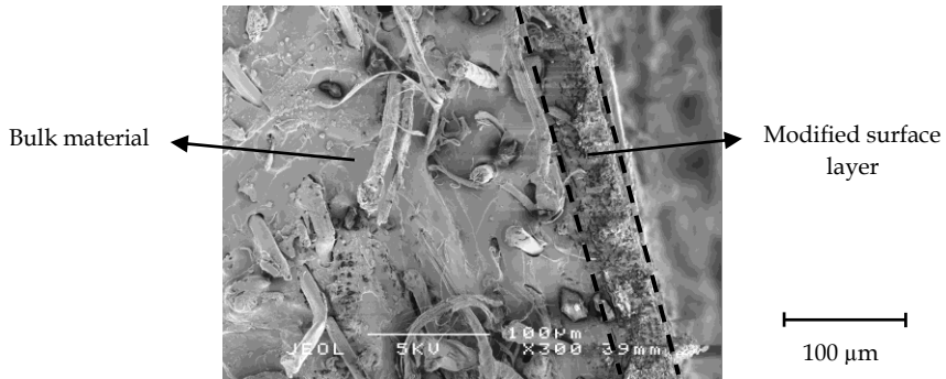
Figure 5.1: The modified surface layer of short-cut aramid fibre reinforced elastomers, shown as a cross-section image.
