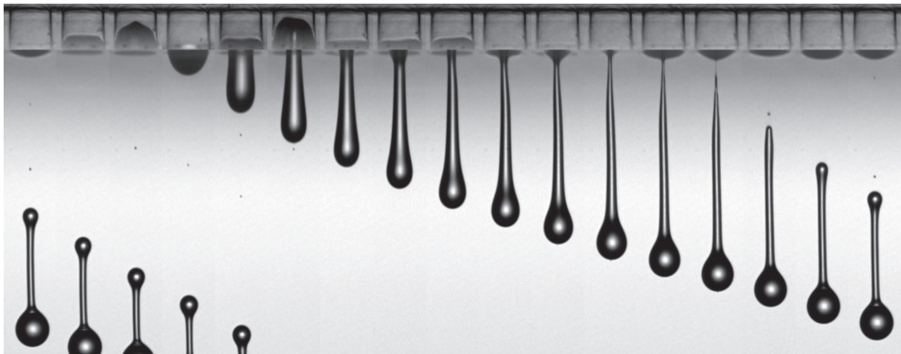
Figure 1.1: Droplet formation from a 30 \mu\text{m} diameter nozzle of the experimental printhead described in Chapter 4. Recorded using 8 ns single-flash stroboscopic imaging with illumination by laser-induced fluorescence (iLIF) [37]. The nozzle and the droplet were imaged at a different focal distance during separate recordings, and were stitched together in this image. Thus, each image of the nozzle and each image of a droplet shows a different droplet formation.
