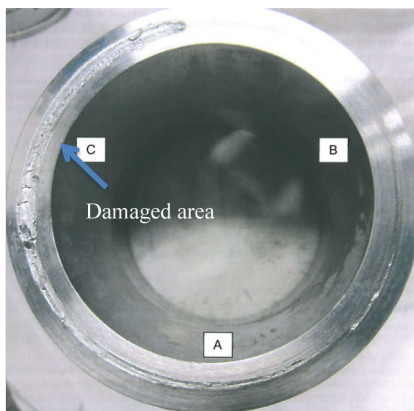
Figure B.7.: Results of the as machined reference test. Surface damage after make-up sliding with API modified. Letters indicate orientation of specimen to match with the counter surface.
