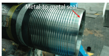
Figure C.1.: Male or "pin" member of a premium casing connection assembly. The pin is connected to a female or "box" member by the thread. At the final moment of assembly the metal-to-metal seal engages ensuring a gas tight connection. Picture: Rob Keeris.
