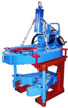
Figure 1.4.: A power tong for assembly of casing connections. The lower part is stationary and grabs the box and the top part grabs the pin and is driven by hydraulics. Picture: Universe Machine Corporation.
