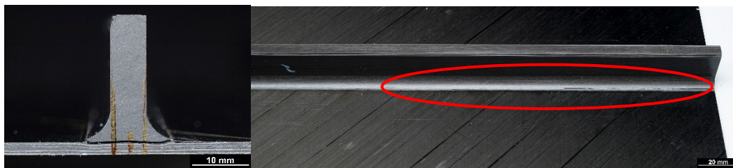
Fig. 3. Close up on the damage in panel 5565.
