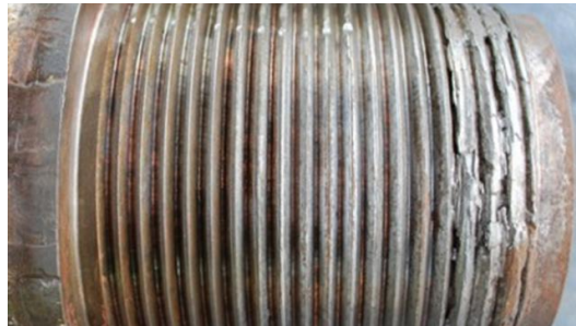
Figure 4.2. Example of a "galled" connection [15].
