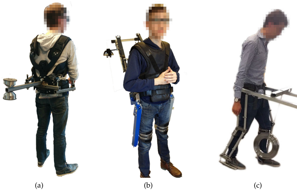
Figure 9: POCs trunk support. (a) Counterweight, evaluated in [20]. (b) Spring, evaluated in [20]. (c) Parallelogram, evaluated in [35].
