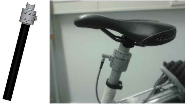
Figure 8, Saddle tube sensor on saddle tube. Superior on the tube sensor a mounting area for the saddle is present.
