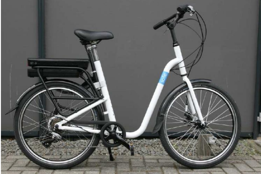
Figure 21, the final design of the SOFIE bicycle with geometric adaptation compared to a standard city bicycle resulting in a higher intrinsic bicycle.
