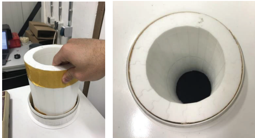
Figure 6.22: The internal Acoustic Black Hole muffler inside the ventilation unit.
