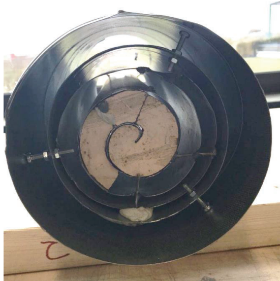
Figure 6.9. The spiral resonator inside the co-axial duct.
