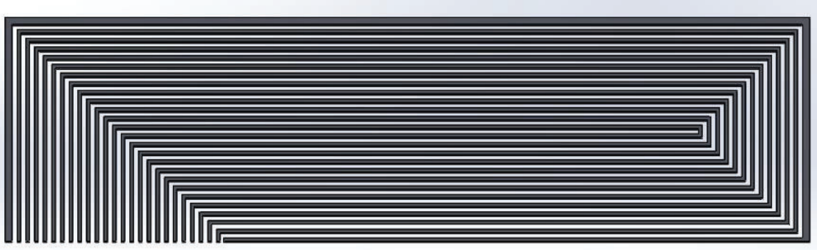
Figure 4.27: Front section view of the long cylinder resonator with 12 Loops.
