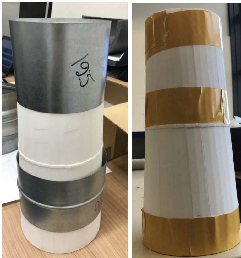
Figure 5.13: The prototype of the internal Acoustic Black Hole muffer.
