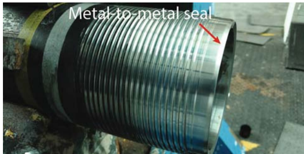
Fig. 1 Male or “pin” member of a premium casing connection assembly. The pin is connected to a female or “box” member by the thread. At the final moment of assembly, the metal-to-metal seal engages ensuring a gas tight connection
